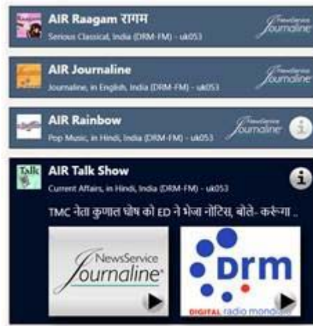
Basic DRM transmission with 3 audio services + Journaline and slideshow (with station logos and Unicode support)
